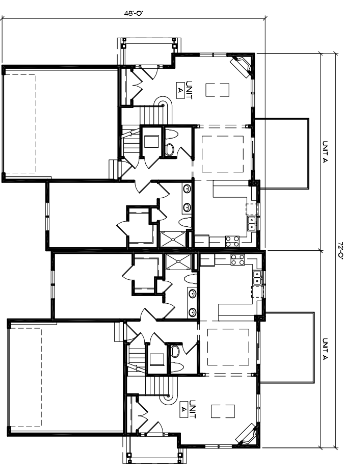
FIRST FLOOR PLAN - 2 UNIT BUILDING (BLDGS. 1, 2 & 4) Scale: 1/8" = 1'-0"
